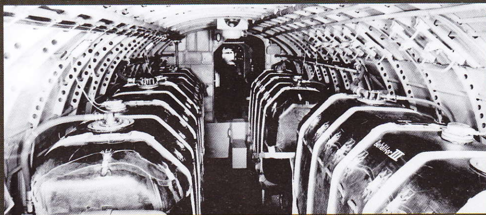
Five additional fuel tanks carrying 1,100 litres (242 Imp Gal.) each were installed allowing up to 14 hours flight time for a range of about 3,860 km (2,398 miles) subject to bomb load. Two additional 625 litre (137 Imp Gal.) tanks could also be carried in place of the bomb load in the ventral gondola.
