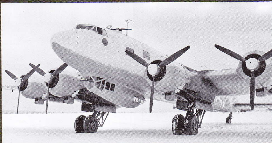
In December 1942, Hitler received armed Fw 200 C-4/U1, 0137, CE+IB, as his new personal aircraft. It had a shorter ventral gondola than the standard Fw 200 Cs in order to leave space for the special parachute seat. Later Dönitz, Himmler, Keitel and Speer also used Fw 200 Cs as their personal transports.
