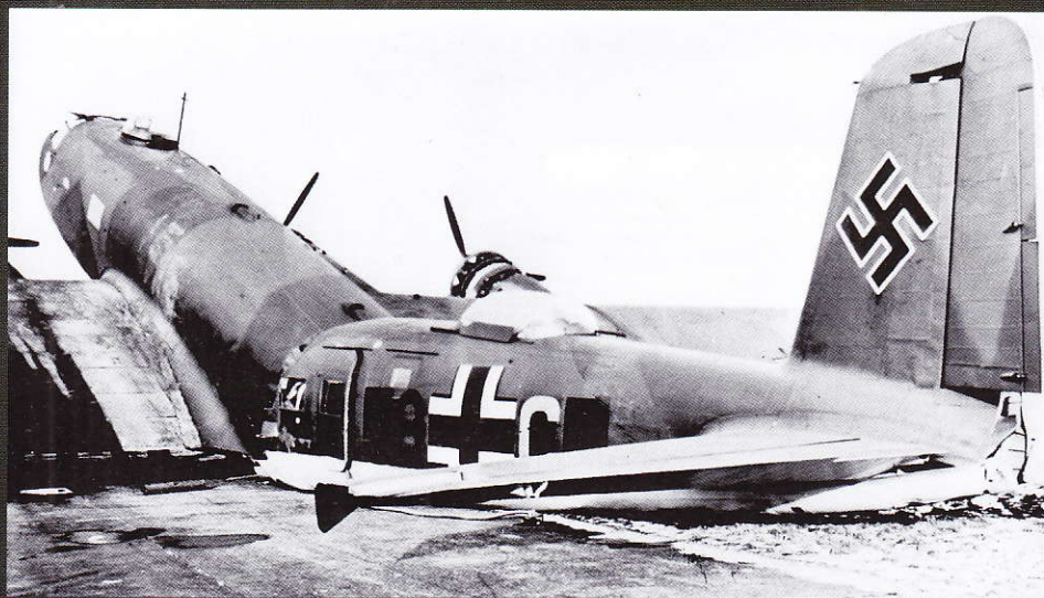
For early Fw 200 C models taxiing fully loaded or with an overload meant there was a high risk of the weak fuselage structure failing just aft of the wing, resulting in a broken back. Surprisingly all aircraft were repaired and restored to full airworthiness by field repair shops.
